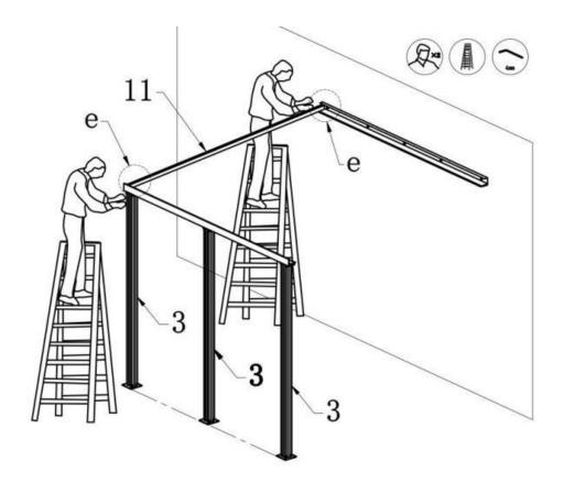
Install the central spars (12), and secure using M6 x 16 hex screws (5). Now install the second side rail (11), again ensuring the threaded holes are on the outside (e). Secure using M6 x 16 hex screws (5).
