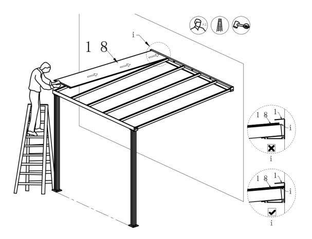
Make sure the polycarbonate panel (18) is correctly positioned on the rails (11, 12) and then use a rubber mallet on both sides of the panel to slot it into the rail grooves. Only a rubber mallet may be used, do not use steel or wooden hammers as the polycarbonate could be damaged.
